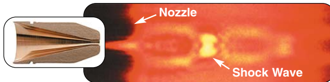
Schlieren image showing density gradients clearly identifies a Mach Disc (shock wave) present in the gas flow as it exits from a traditionally manufactured laser nozzle.
